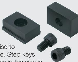
Hardened vise keys are used to align your Kurt vise to your milling machine table. Step keys are used when the keyway in the vise is different than that of the machine T-slot. Standard keys are used when they are the same width.
